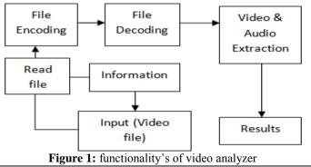
Next Generation Computing Technologies Sankara College Of Science And Commerce The basic Functionality of video analyzer is diagrammatically represented below: Analyzer read an input video file from Information (knowledge base) and makes the video file Encoding and Decoding process, finally extract the information's from the particular video file and provide the results. The result contain, type of the video file, frame per second etc.,
